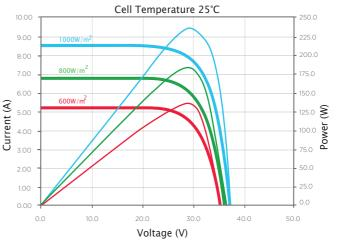
Current, Power vs. Voltage Characteristics of RNG-240P
