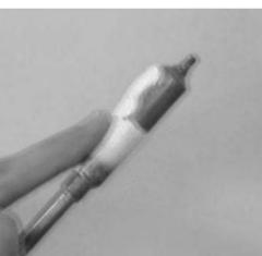
**Step 2:** Carefully insert the heat pipe into the copper sleeves located inside the manifold.
