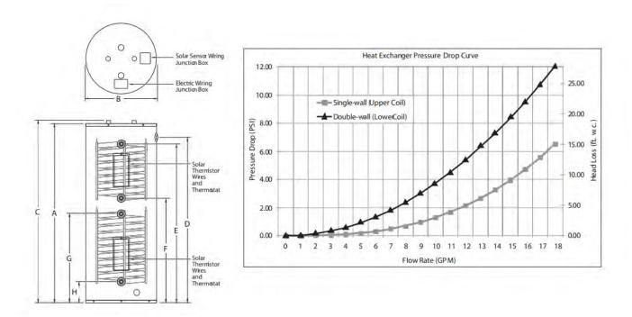
All water heaters are certified at 300 PSI test pressure (2068 kPa) and 150 PSI working pressure (1034 kPa). All potable water and electrical connections are ¾"NPT (19mm) on 8"(203mm) centers. All models are UL listed.
