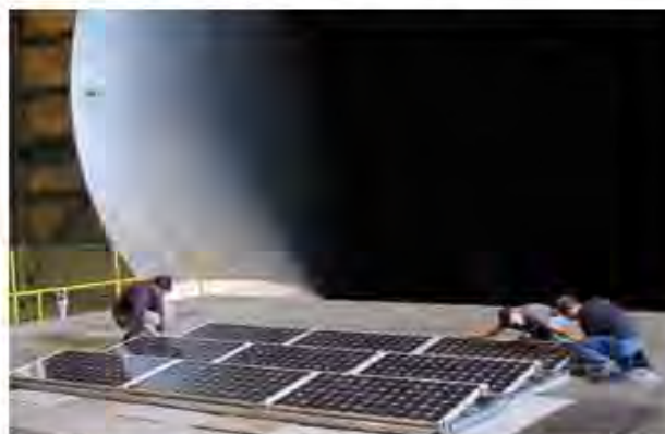
The POWER-FAB CRS has been full scale wind tunnel tested and qualified.
