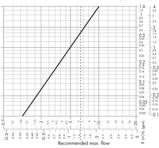
The maximum recommended speed of the fluid in the piping is 4.2 ft/sec, which is equivalent to a flow rate of 6.5 gallons per minute.
